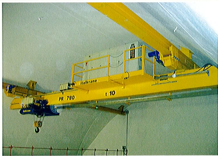
Gru a ponte monotrave sospesa per Laboratorio Ricerca Nucleare - Portata 10 t Suspended Bridge Crane for Nuclear Field - Capacity 10 t
