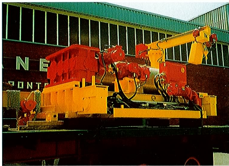
Carrello argano da t 60 con braccio ausiliario Winch crab of 60 t with auxiliary jib
