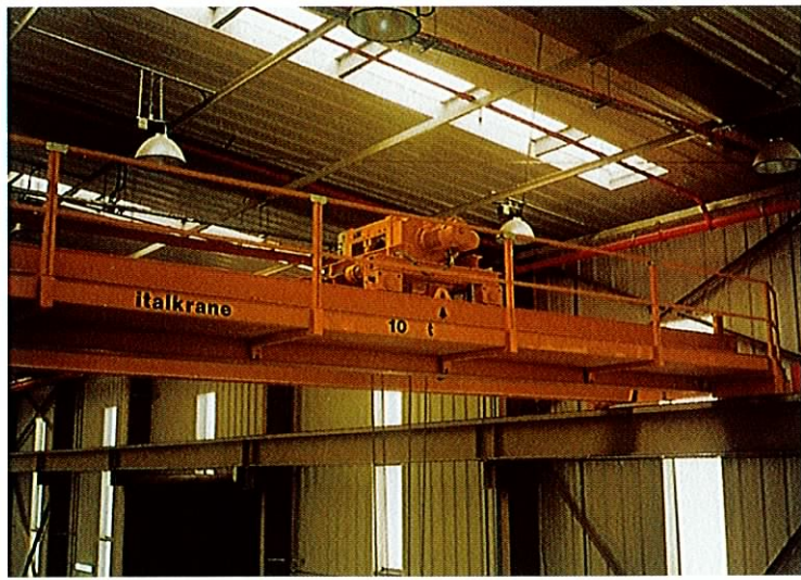
Gru a ponte con carrello argano Portata t 10 - Scartamento m 16 - Alzata m 8 Double-girder bridge crane with winch crab Capacity 10 t - Span 16 m - Vertical path 8 m
